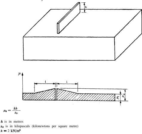
$k = 2 \text{ kN/m}^3$   $\mu_1 = 0.8$  l = 2hRestrictions:  $0.8 \le \mu_3 \le 2.0$  $5 \text{ m} \le l \le 15 \text{ m}$
