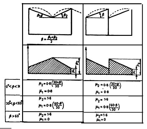
• For asymmetrical simple Pitched roofs, each side of the roof shall be treated as one half of corresponding symmetrical roofs.
