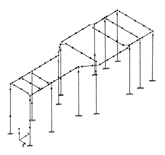
Fig. 3 Space Frame Model of the Foundation Shown in Fig. 1
