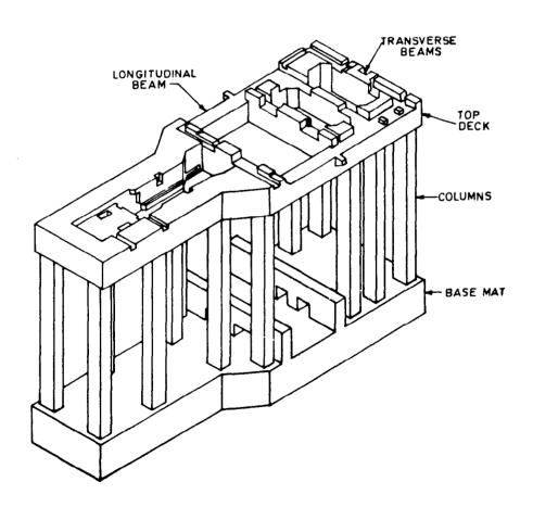
Fig. 1 Typical Framed Foundation for a Turbo-Generator
