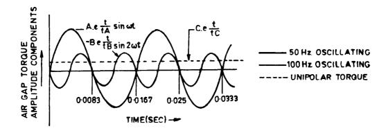
Fig. 4 Short-Circuit Moment Diagram
