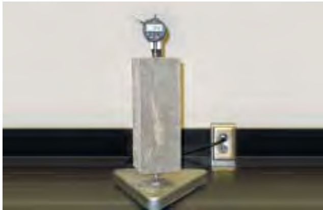
Length Comparator with specimen in place
