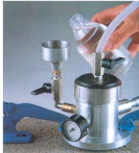
In-situ Water Permeability of Concrete
