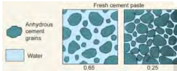
Schematic representation of two fresh cement pastes having a water/cement ratio of 0.65 and 0.25.
