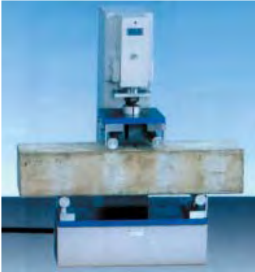
Flexural testing of concrete beam mould
