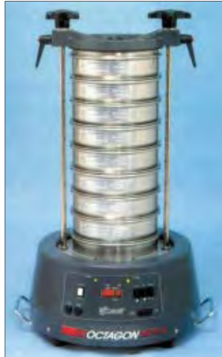
Set of Sieves assembled for conducting Sieve analysis.
