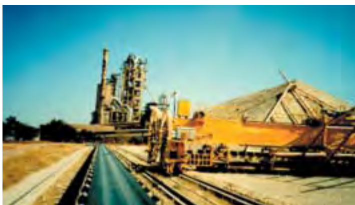
Reclaimer for homogenization of crushed limestone.
