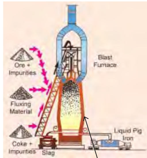
Refractory concrete made with High Alumina cement is used as refractory lining in furnaces and fire pits.
