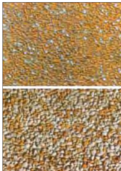
Exposed aggregate architectural concrete by making use of Surface Retarders.
