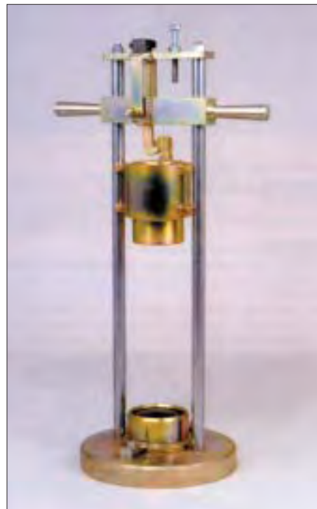
Aggregate Impact Value Apparatus.
