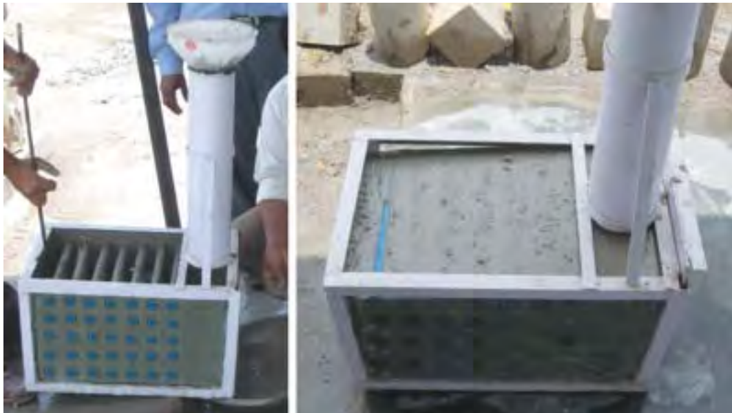
Detail of the Fill-Box empty and filled with concrete. Courtesy : Hindustan Construction Company
