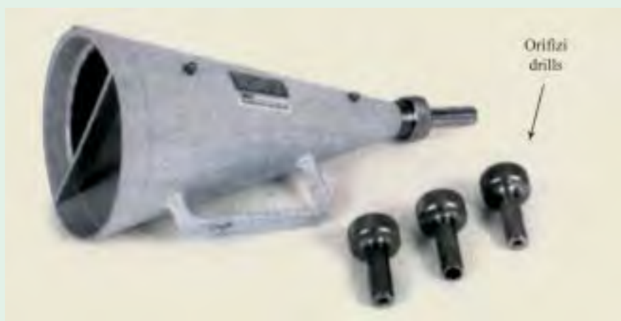
Fig. 5.5. Marsh cone viscometer with attachments, 6 mm, 8 mm and 11 mm.
