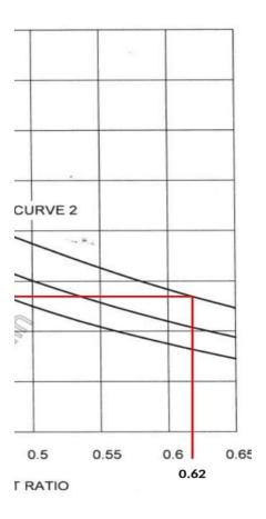
this aggregate volume are given in Table 5 for a nentitious materials ratio of 0.5, which may be ther ratios, the proportion of volume of coarse otal aggregates is increased at the rate of 0.01 c-cement/cementitious materials ratio by 0.05 and 1 for every increase in watercement ratio by 0.05.
